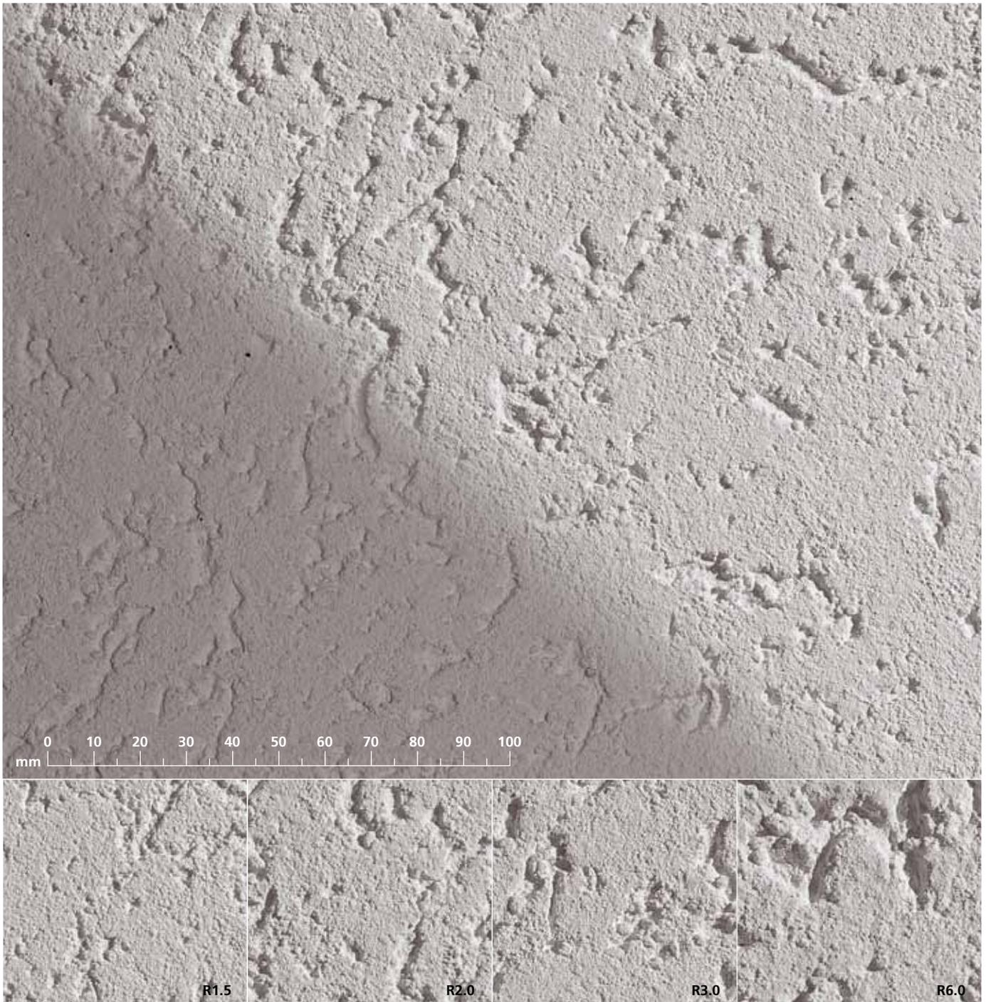
An attractive drag finish for synthetic renders with the appearance of a scratch plaster. The rilled texture helps to give the finished substrate a flatter and more even appearance.
