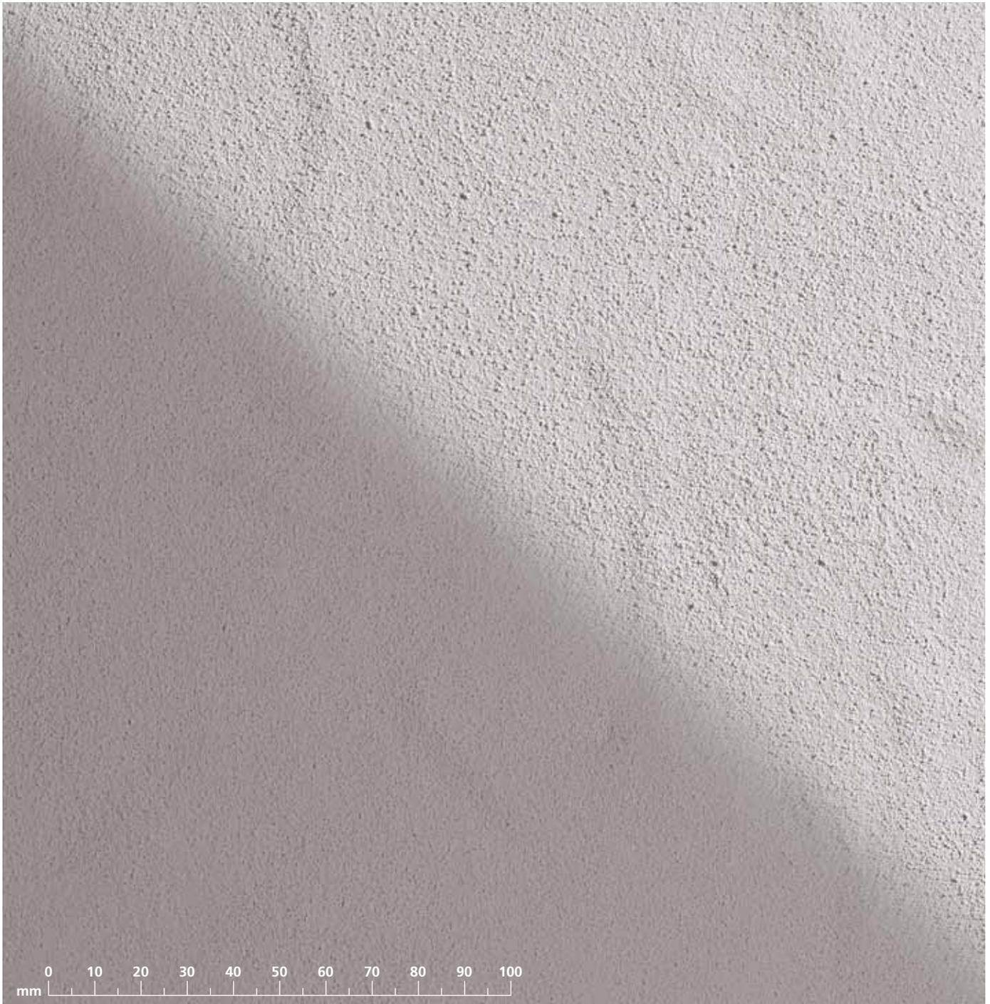
If a unique, bespoke facade finish is required, MP renders are the ideal solution. The material can be rubbed up to give a near smooth texture or provide a variety of textures for the facade.
